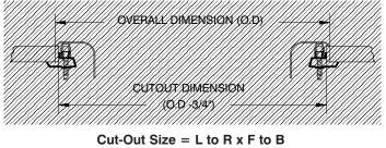
Standard Mounting Clips Fit Countertops Over 7/8" & Up To 2" Thick.
