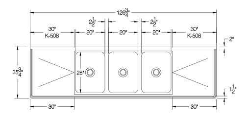
K-23A Welded / Crated Set-Up (Unit Fully Welded)
